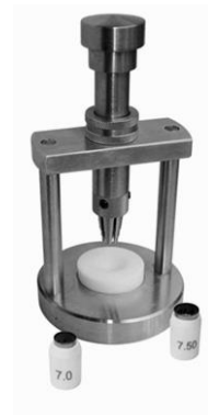
RLH - 189 ENDOTHELIAL PUNCH SPRING RECOIL USED FOR DIFFERENT SIZED TREPHINES
